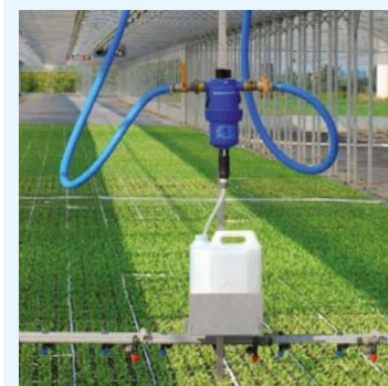
Proportional dosing unit assembled directly on the irrigation boom .
