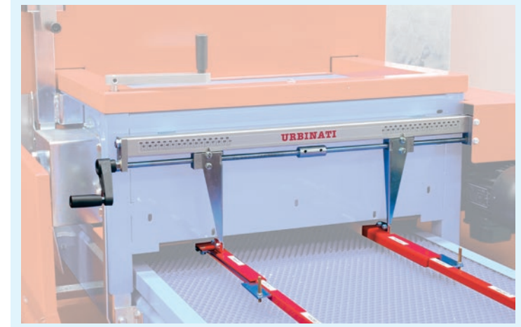
Quick self-centring guides adjustment system.
