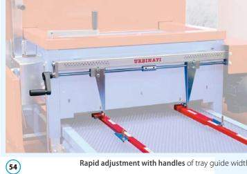
Rapid adjustment with handles of tray guide width.
