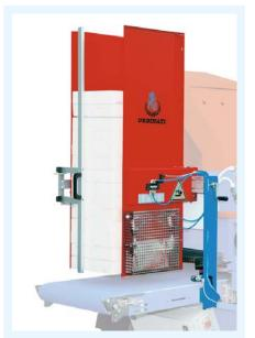
Electropneumatic denester with nr. 2 movements, adjustable with a single handle; for polystyrene trays and carrier.
