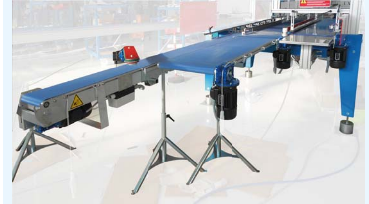
With the 3 axis transplanting selection , the machine can be set with two destination areas: one for trays and the other one for pots.
