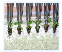
The exclusive flat profile of the needles and the closing system allow an excellent grip of the plug even with weak-rooted plants.
