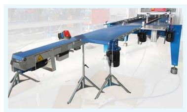
With the **3 axis transplanting selection**, the machine can be set with two destination areas: **one for trays and the other one for pots**.
