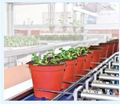
**Pot positioning** on the belt with cylinders (diameter pots from 9 to 20 cm).
