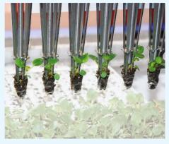
The exclusive flat profile of the needles and the closing system allow an excellent grip of the plug even with weak-rooted plants.
