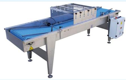
The SUB-IRRIGATION machine is mainly recommended when a uniform watering is needed or when the watering from above is not enough.
