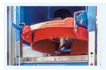
Cutting system and product aspiration with rotating blade. It ensures a **precise cut** and an excellent cleaning of the trays without any residual leftover.
