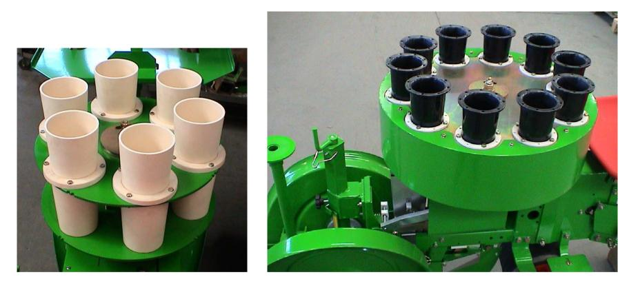
Carousel of plant distribution with 6 or 10 cups on crawling steel plate (option)
