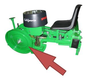
The plate of falling pipe has the function to help plants to stay straight when they fall in to the shoe.
