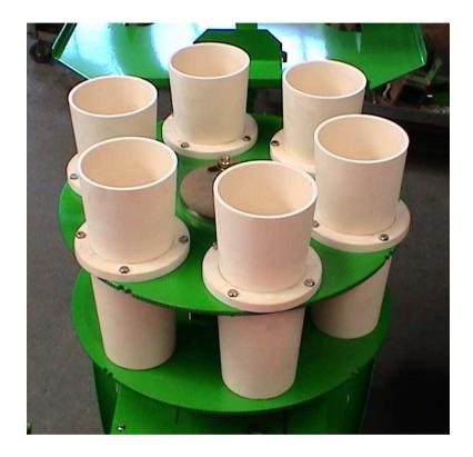
Carousel of plant distribution with 6 cups on crawling steel plate (option)
