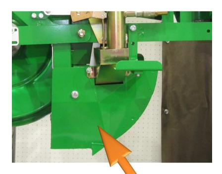
The shoe create the furrow where machine will put plants. It's made by hardened boron steel.
