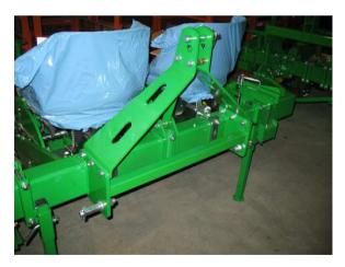
Standart three point hitch for machines till 3/4 units frame L=2,45m max.
