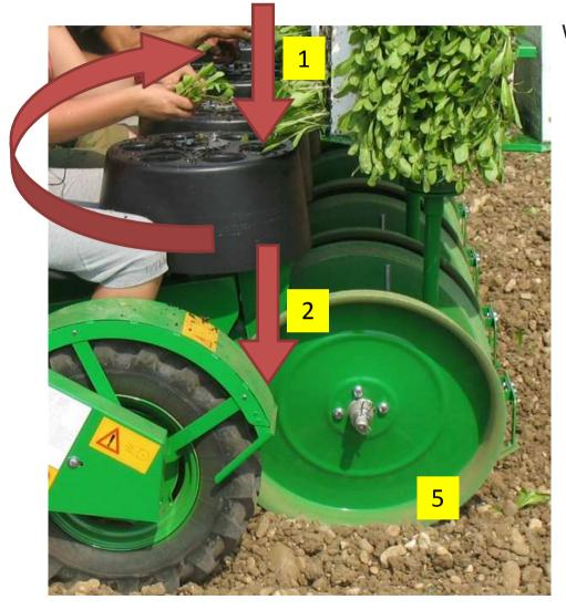
When cups of rotating carousel run over falling pipe [1] they open and plants get down throught falling pipe [2] in the shoe [3].
