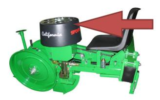
The carousel is made by teflon-nylon material:
