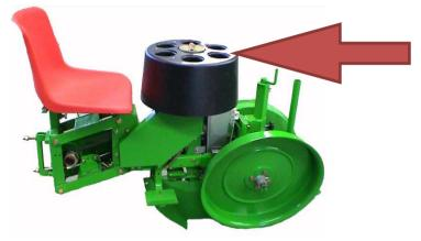
The carousel is made by teflon-nylon material:
