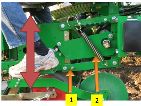
The parallelogram [1] allows the planting unit to follow the contours of the land.
