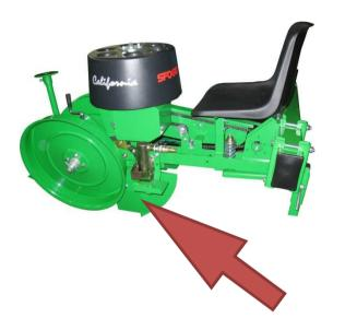
Kicker has the important function to push plants in the furrow made by the shoe. It is self-cleaning, in case of stones that go inside the shoe it automatically push them out.
