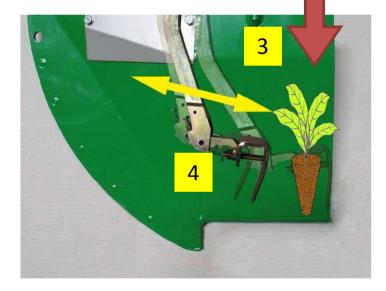
Inside of the shoe there is a kicker [4] that push plants in the furrow made by the shoe. Back wheels regulate planting depth and close the furrow and press the soil at sides of plants.
