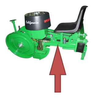
The floating frame [1] allows the planting unit to follow the contours of the land.
