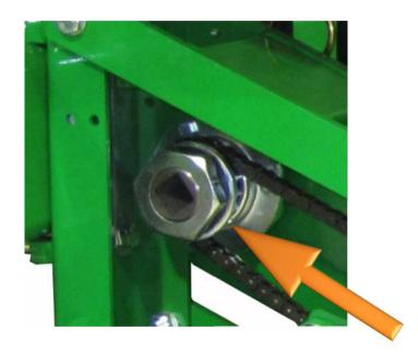
Planting unit has a security clutch: in case of objects/stones/etc that block the carousel rotation, it intervenes and doesn't allows breakage.
